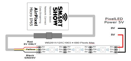
The 3-wire Waterproof cable has the following connections:
