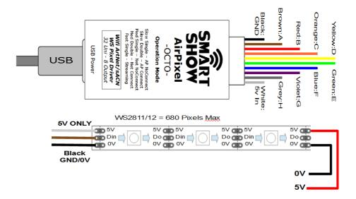
The multicore output ribbon cable has the following connections:
